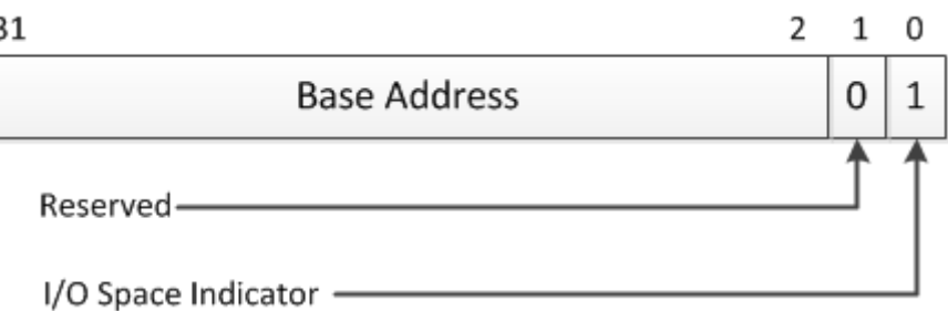
Figure 6 BAR That Maps to CPU I/O Space Format
